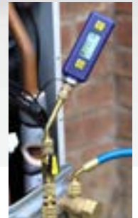
5° bend ¼ flare female connector connects directly onto the system allowing for a more accurate reading
